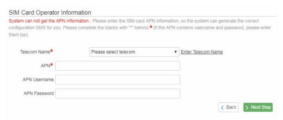
3.7 Click Next Step, OVERSEE gives the configuration SMS to you. Please copy it and send it to the gps device, after you receive reply from the gps device, it should be online.
